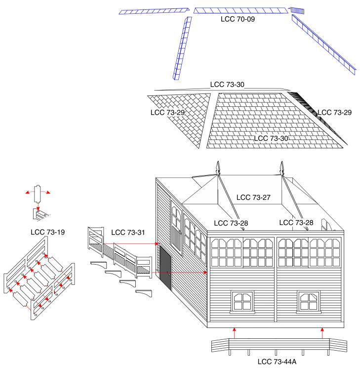
Glue LCC 73-28 into the slots in LCC 73-27. Glue the roof panels to the roof support assembly. Make sure this is done on a flat level surface to ensure the roof is straight. The support structure is designed to be slightly lower than the roof panels therefore do not put a lot of pressure on it from the top or it will come apart. Finally finish the roof with ridge tiles (LCC 70-09) by gluing them on top of the joints and trimming where necessary.
