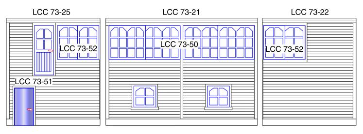
When the laminates finish drying glue the windows and doors into the openings. Cut out the door handles from LCC 73-51 and glue them to the both doors. There is no particular pattern the windows have to follow regarding the sliding part. Prototypes of this signal box had the sliding windows both at the near corner position as well as mixed or on the far side of the corner.
