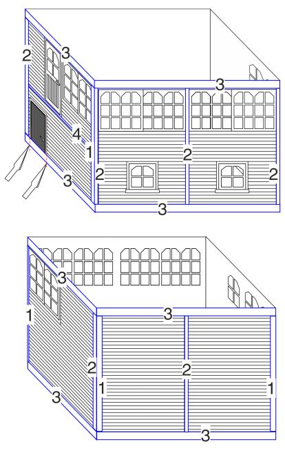
As a general rule of thumb the thicker strip (1) should be glued onto the "end grain" of the corner followed by the thinner strip (2) on the other side of the corner. Front and back vertical strips in the middle should be thinner. Bottom and top strips are the thickest. On the side with door a section needs to be cut out to allow for the door. Final piece (4) should be glued just below the upper floor door.
